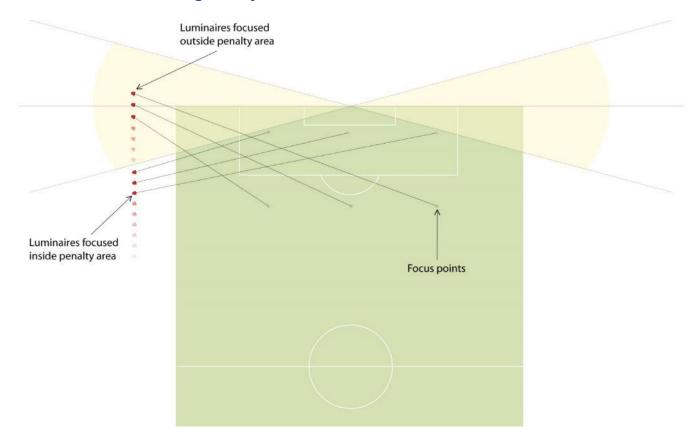
As regards players in the penalty area, the discomfort glare produced by a linear run of luminaires is considered to be within an acceptable level if the luminaires' focus points are such that players can stand in the penalty area and look towards the corners without hindrance.
