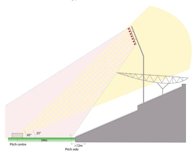
Stadium structures should not impede the luminous flux of the pitch lighting system and cause shadows to be cast on the surface of the pitch. Care should be taken to ensure that the luminous flux projection lines to the pitch surface are completely clear.
