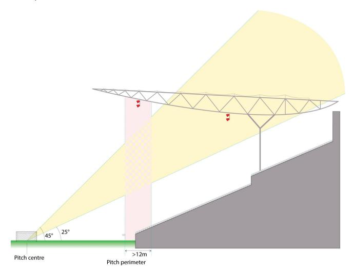
If the stadium design or existing installation requires luminaires to be positioned within a lateral distance of 12m of the perimeter of the pitch, or if the vertical illuminance requires improvement, a second linear run of luminaires should be used to achieve the required vertical illuminance around the perimeter of the pitch.
