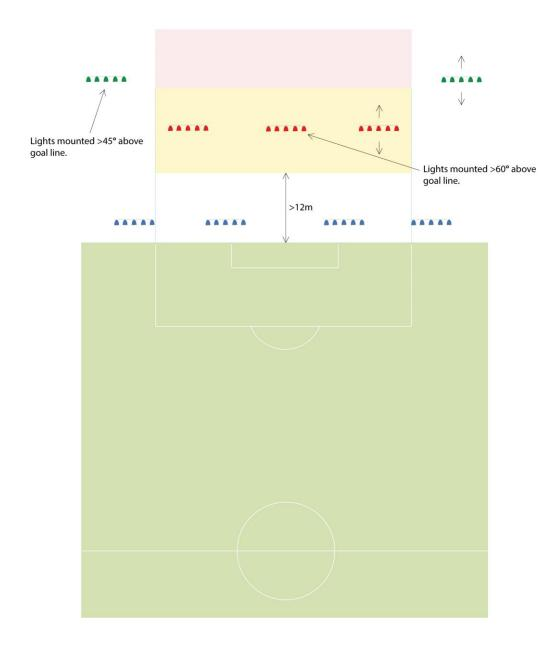
Luminaires positioned behind the goal and parallel to the penalty box as indicated in Section 6.8 should be mounted more than 60° from the goal line when in line with the penalty area, as indicated in the diagram above.
