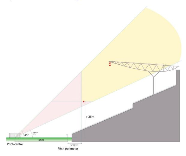
The luminaires should not be mounted less than 25° or more than 45° above the centre of the pitch.
