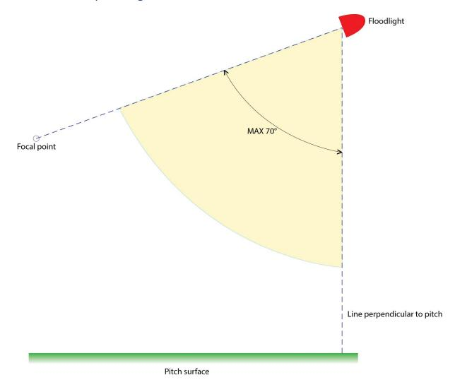
In order to avoid discomfort glare being experienced by players and officials, a general rule during the design process is to ensure that luminaires' focus point angle is no more than 70° from the line perpendicular to the pitch, as in the diagram above. This is a good general guideline, but it will not always be possible owing to the constraints of the stadium's design.
