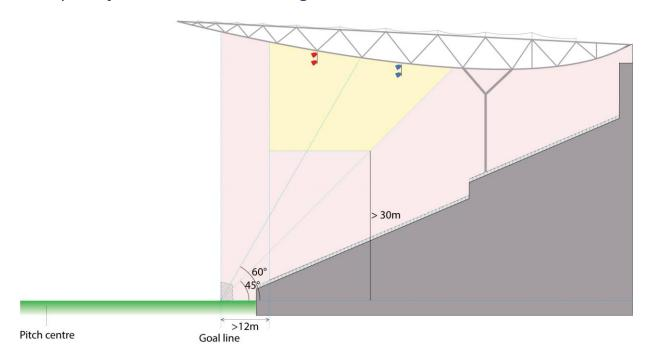
In order to avoid discomfort glare being experienced by attacking players looking towards the goal, additional provision is made by increasing the installation angle of luminaires directly behind the penalty area (as shown in the diagram above).
