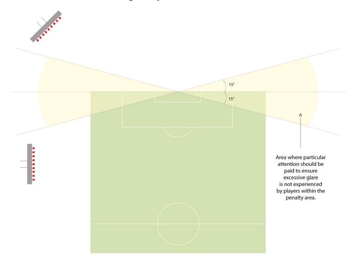
When pitch illuminance is provided by means of corner columns or towers with multiple luminaires in a group (as is generally seen in columns and towers), the luminaires should not be mounted within 15° of either side of the goal line (see diagram above).
