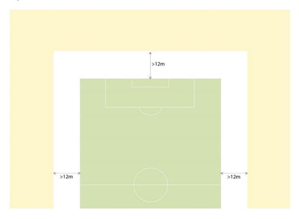
In order to achieve the required vertical illuminance around the perimeter of the pitch, the luminaires should have a mounting position with a minimum lateral distance from the pitch perimeter of greater than 12m.
